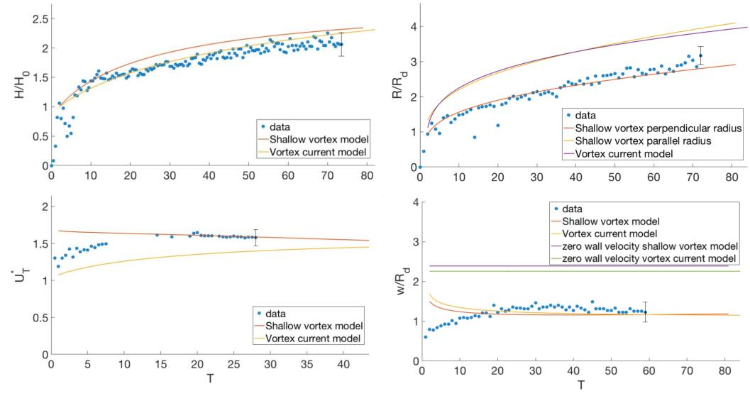
**Figure 3: Comparison of the experimental data with the new time-dependent** model for the vortex depth H, radius R, and current velocity U<sub>T</sub>, width w.
