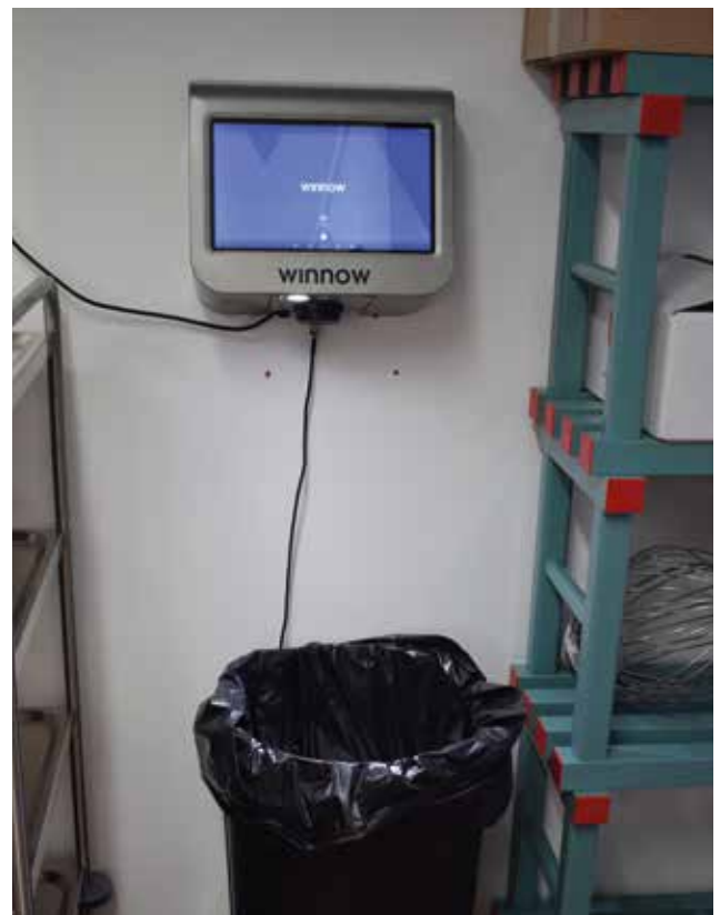
Food waste is hard to measure and hard to manage. The Hall has installed a Winnow food waste system which makes it quick and easy to record exactly how much food is being wasted through smart technology attached to our kitchen food waste bin.
